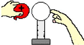
At this point, there is a movement of electrons. Electrons move
