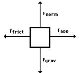
The free-body diagram above depicts four forces acting upon the object. Objects do <u>not</u> necessarily always have four forces acting upon them. There will be cases in which the number of forces depicted by a free-body diagram will be one, two, or three. There is no hard and fast rule about the number of forces that must be drawn in a free-body diagram. The only *rule* for drawing free-body diagrams is to depict all the forces that exist for that object in the given situation.
