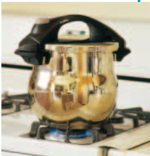
This cooker is sealed so that the volume is constant. Pressure increases in the cooker as temperature increases.
