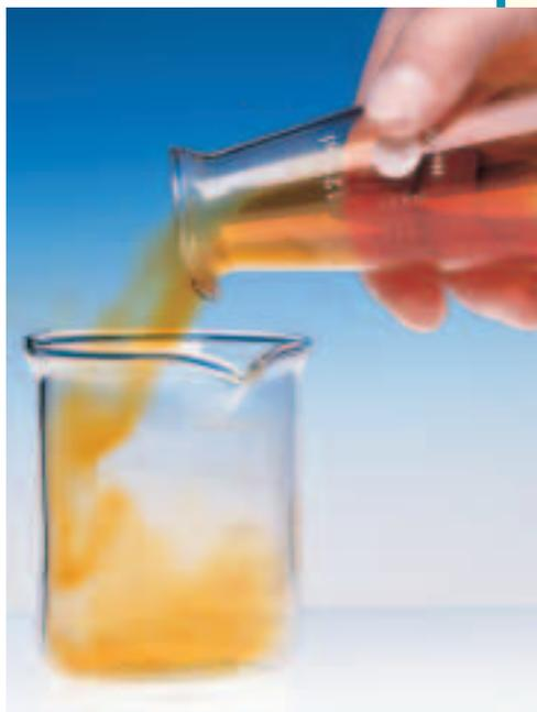
The density of a gas can be used to identify it. This gas is denser than air and can be poured from one container to another.
